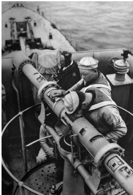
Figure 1. Coincidence rangefinder of the Polish Destroyer ORP Witcher (1935).
